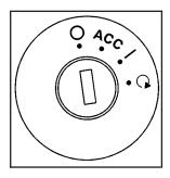
With the key in the ignition switch, you can turn it to four different positions. A warning tone will sound if you open the driver's door when the key has not been removed from the ignition.
